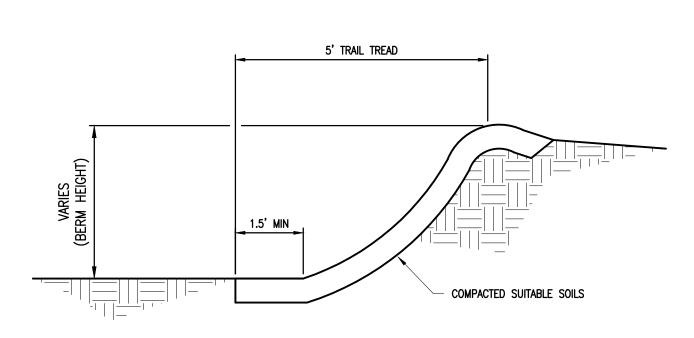
9 SECTION "C" BERM ELEVATION
